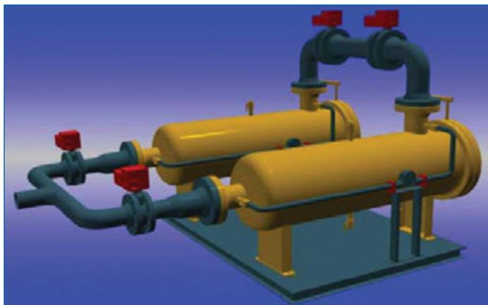
Typical duplex configuration for Condensate CRUD removal
