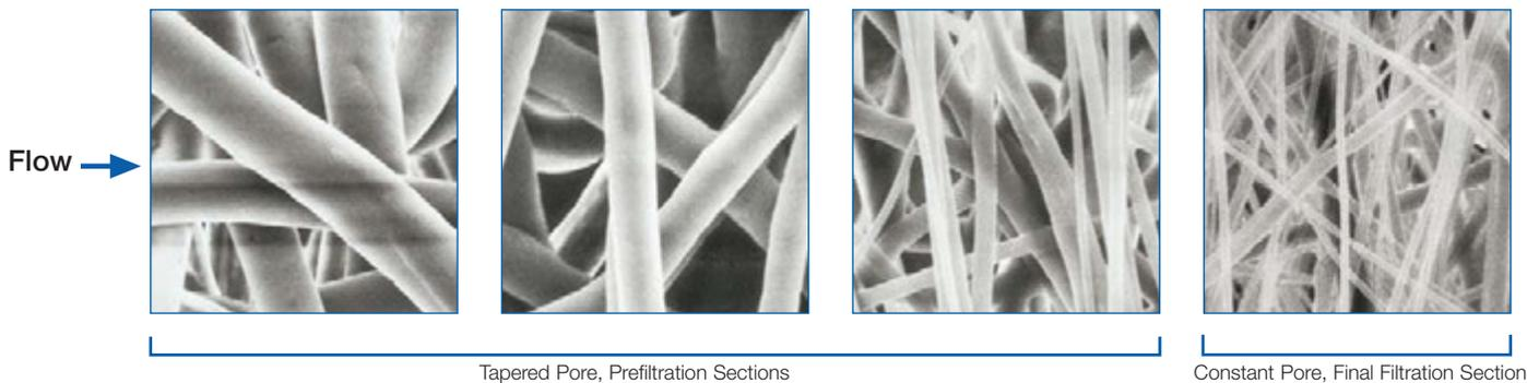
Sample sections of Ultipleat High Flow filter medium at 500X magnification
