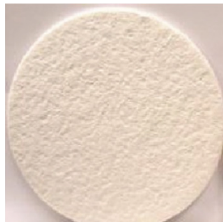
An unused VRF medium.
