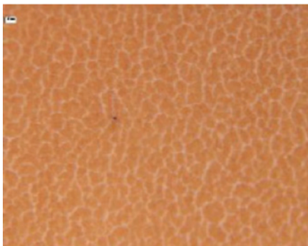
This photomicrograph shows varnish material on an analysis membrane (0.45-micron porosity) at 100x magnification.
